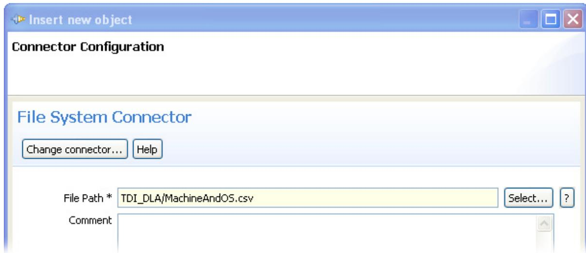
Figure 4 - Configure ReadCSV (04\_ConfigureReadCSV)
