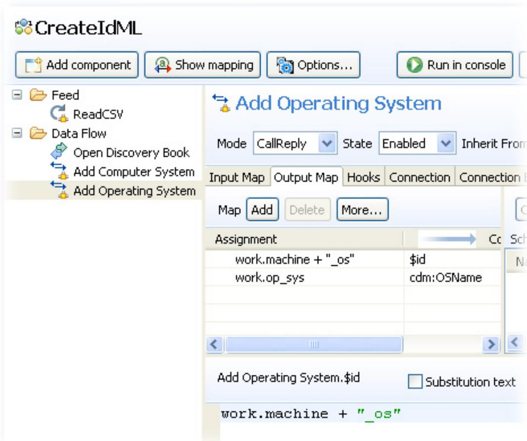
Figure 15 - Output Map for Operating System (14\_AddOS)
