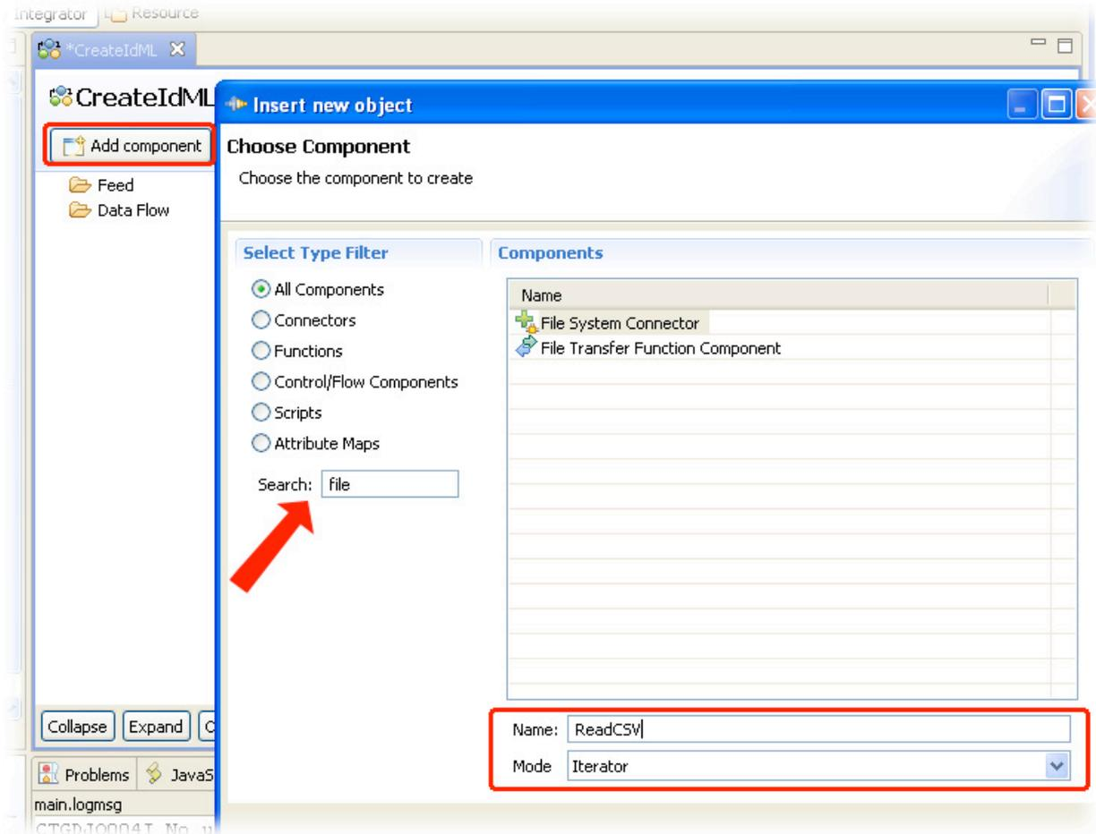
**Figure 3 - Add ReadCSV Connector (03\_ReadCSV)**
